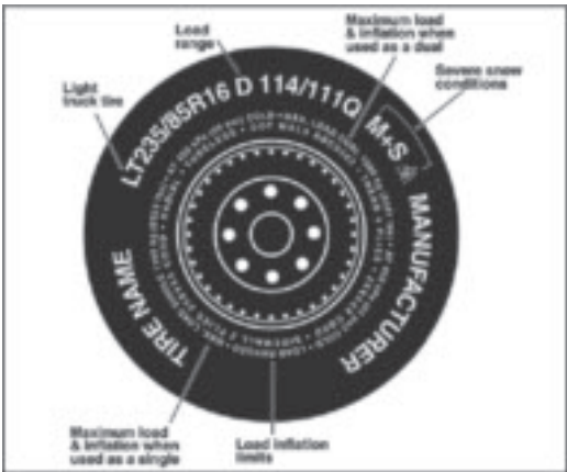
Figure 4: Typical Light Truck Tire Markings
