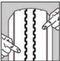
Shoulder wear (have inspected)
