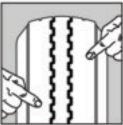
Shoulder wear (have inspected)
