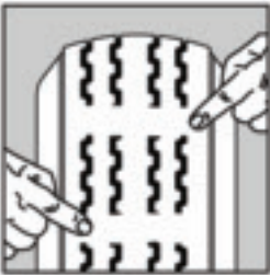
Exposed tread bars (replace)
