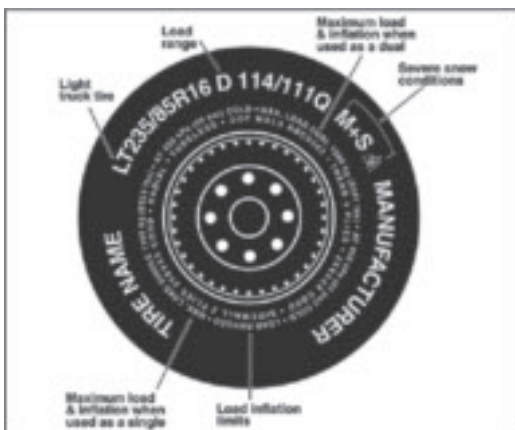
Figure 4: Typical Light Truck Tire Markings
